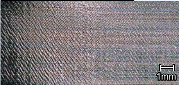
Worn / Cloudy surface
