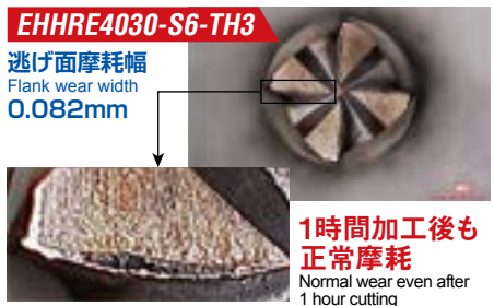
図 荒加工後の摩耗状態 Figure : Wear condition after roughing
