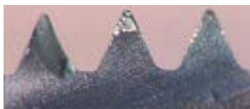
従来品 10穴加工後 Conventional after threading 10 holes.
