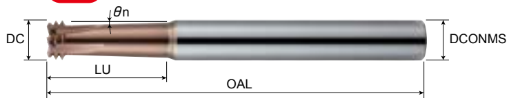
不完全山数: 1山 1 incomplete thread and 2 complete threads
