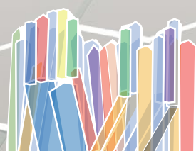
Conventional CVD inserts Grain size and growth direction are uneven.
